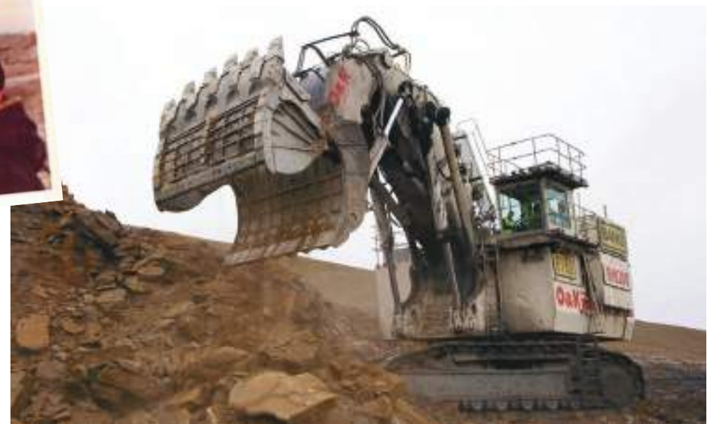
THE LARGEST HYDRAULIC EXCAVATOR IN BRITAIN - THE TEREX O&K RH200: Our first excavator was hired and it could lift 2.5 tonnes. Our first RH 200 carries a bucket capable of loading 50 tonnes each lift. It will load a CAT 785 dump truck in three lifts. To keep it working at it's very best, 60 different engineers have worked on it over the past four years.
