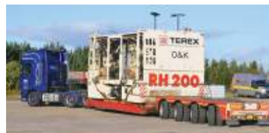
RH200 DELIVERY: Weighing over 500 tones, this piece of kit is so large it had to be stripped down into individual parts and transported to site in 18 separate loads
